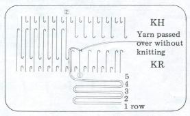
①Set the carriages as the diagram and knit a row over the needles in E position.
