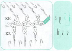
R-2)-b Knit 1 row. Take the loop of the first stitch on KH and put it onto the second empty needle on KR side. (By operations (a) and (b) 1 stitch is increased.)
