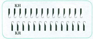
Cast on stitches using a cast-on thread for full needle rib. Hang on cast-on comb and weights.
