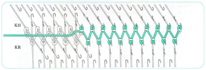
4 Knit 1 row. For the second time read the stitch measure scale and push up the corresponding needles to E position. Knit the 3rd row.
