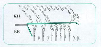
B-3) Knit 1 row. The newly increased needles knit. Transfer the stitches on KR to KH. (5 stitches have been increased).
