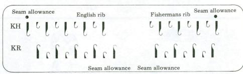
② Since the pattern is English rib or Fishermans rib, begin with 1 round of circular knitting for the finished edge. Set the Slide lever at 1 and knit the length of the collar adjusting the tension dial by referring to the tension adjustment chart.
