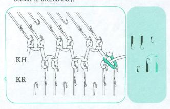
③ Knit until next increase. Take the loop of the first stitch on KR and put it onto the 2nd empty needle on KH
