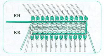
Repeat  $1\sim 4$ . Before you start to knit the garment, make a sample swatch and see if both beds knit to the same tension. If they do not, adjust the tension dial on KR carriage.
