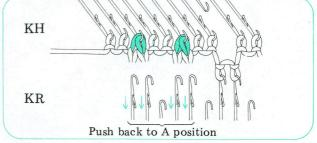
★ When fewer needles on KR are used, decreases are worked in the same manner by transferring stitches onto the corresponding needles on KH.
