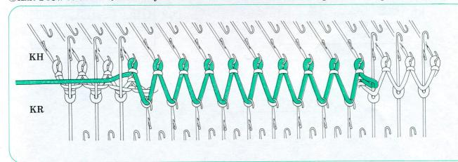
⑤Turn the racking handle 1 pitch to the right (the racking indicator is at 4). At the opposite side of the carriage, place the needles not to be knitted on KR to E position, and the needles to be knitted on KH to E position. Knit 1 row to the right. Pass the yarn behind the stem of the innermost non-knitting needle on KR and knit a row to the left.
