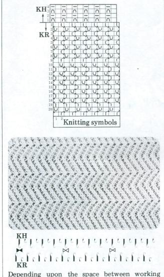
Depending upon the space between working needles, you can produce a fabric from bulky to light and open. By placing some needles into A position even heavy yarns can be knitted, but fine yarns are very effective if used in this way. Try it out with lurex or lame and you will be suprised what an elegant evening dress you can make!
