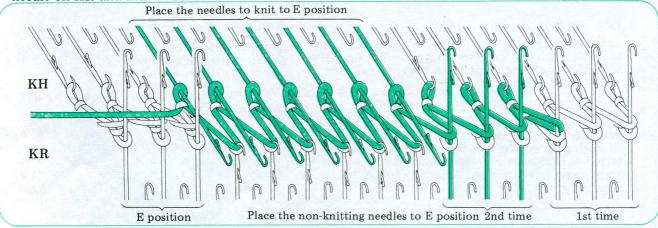
Turn the racking handle 1 pitch to the left (racking indicator at 5) and repeat the above to shape your garment by partial knitting.
