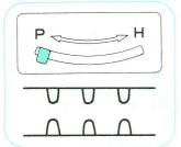
The needles on both beds are exactly opposite each other. When this is the case, NEVER knit using all needles in working position.
