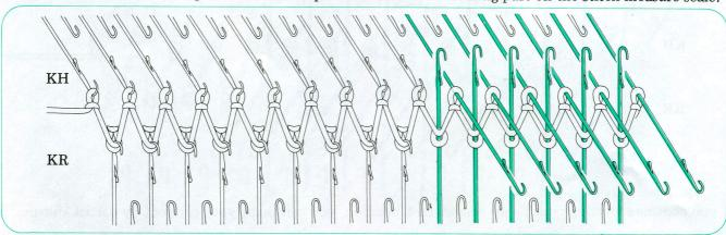
③ Knit 1 row from left to right. Pass the yarn from behind the stem of the first needle in E position and push out the relevant needles on KH and KR to E position, at the side opposite to the carriage.
