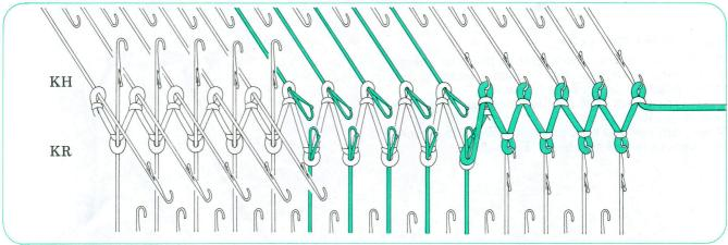
By pushing back the needles to D position you can increase the number of stitches working and shape your garment by partial knitting.
