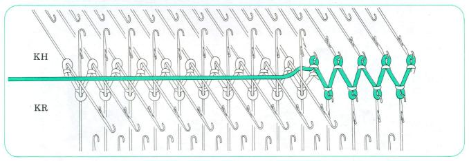
④ Knit 1 row. Read the stitch measure scale and push back the corresponding needles to D position. Knit the 3rd row.
