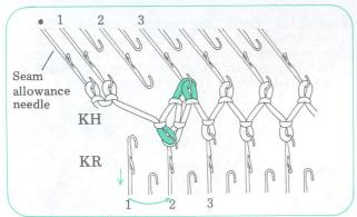
3 Move in 2 stitches on KH to the vacant 2nd needle using a 1 x 2 transfer tool.
