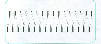
Place the empty needles in B position. (Keep 2 end Ns on KH). Return P to H.
