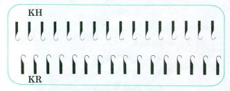
Begin knitting the same as for full needle to rib using a cast-on thread. Hang cast-on comb weights.
