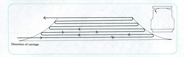
$\bigstar$  To work partial knitting on racking patterns, if the non-knitting needles on KH and KR are placed in E position, they cross one another and the KR bed cannot be racked. So the following method is adopted.
