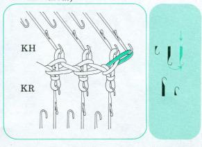
L-1)-b Knit 1 row. Transfer the loop of the stitch on KH (as there is no loop on the edge stitch on KR) onto the vacant needle on KR. (By operations (a) and (b) 1 stitch is increased.
