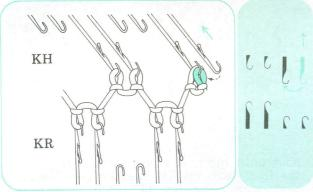
②Knit until the next decrease. Transfer the first stitch on KH onto the first needle on KR. Push back the empty needle to A position. (1 stitch is decreased.)
