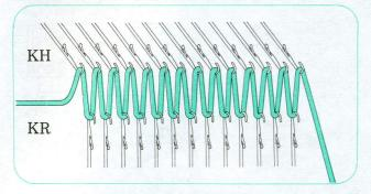
Shang the cast-on comb Hang on the cast on comb same as for  $1 \times 1$  rib.
