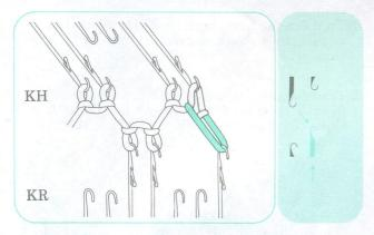
② Knit until the next increase. Transfer the loop of the first stitch on KR to the first vacant needle. (1 stitch is increased.)
