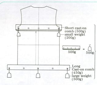
After the armholes are finished change to the short cast-on comb.
