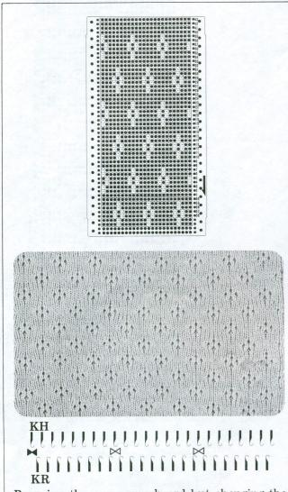
By using the same punchcard but changing the needle arrangement on KR, you have different kinds of patterns. The photographs of variations No.1 to No.3 show more and more needles placed in A position, resulting in a thinner fabric. Plain yarns are recommended. This type of fabric is very suitable for sweaters, one piece dresses, etc.
