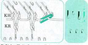
R-3)-b Knit 2 rows, Take the loop of the edge stitch on KH and transfer it onto the empty needle on KR. (By operation (a) and (b) 1 stitch is increased.)
