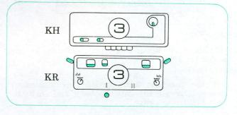
$\star$ For 5 x 5 rib be sure to set the Slide Lever at I.
