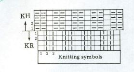
1 Needle arrangement Set the racking indicator on No.5 and the half pitch lever at H, then arrange the needles in B position.
