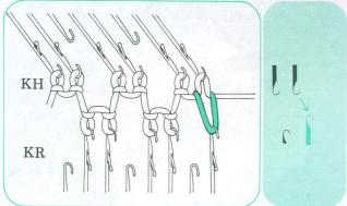
②Knit 1 row. As there is no corresponding stitch on KH side, take the loop of the newly made stitch on KR and transfer it onto the next empty needle. (By operations (1) and (2) 1 stitch is increased).
