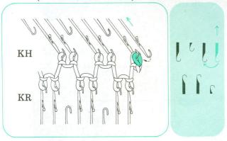
②Knit until the next decrease. Transfer the edge stitch on KH onto the edge needle on KR and push back the empty needle to A position. (1 stitch is decreased.)
