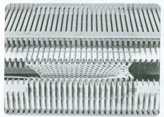
U-style knitting is tubular knitting with one side open. It is useful when working a design which requires a width of more than KH 200 stitches, also for waste knitting to finish ribbed garments, as the stitches can be clearly distinguished by this method.
