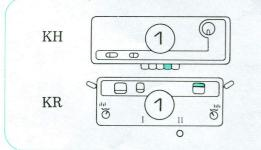
① Move the carriage to the right  $\rightarrow$  The needles on KH only knit.
