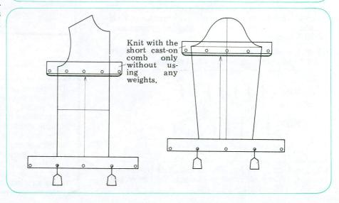
①Changing the Knitleader setting for stitch measure scale and the regulator stitch measure scale (when original gauge is 40 stitches = 10 cm).
