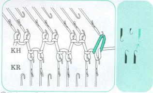
4 Knit until the next increase. Take the loop of the first stitch on KH and transfer it onto the next empty needle. (1 stitch is increased.)
