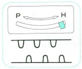
When the needles are at half pitch, it is possible to knit on every needle (full needle rib).
