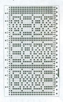
★Thread 3 different coloured yarns into the colour changer feeders (Nos. 2, 3 and 4) and with the No. 1 button pushed in, thread the yarn feeder with the basic colour.
