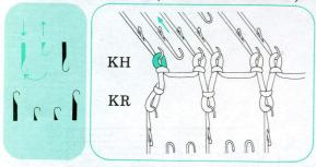
R-2) Knit until next increase. Transfer the first stitch on KH to the next outer needle. Push back the empty needle to A position.
