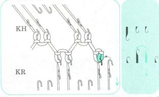
4 Knit until the decrease. Transfer the first stitch on KR onto the first needle on KH. Push back the empty needle to A position(1 stitch is decreased.)
