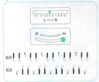
In order to have the yarn cast on alternately on the hooks change the setting as illustrated below.
