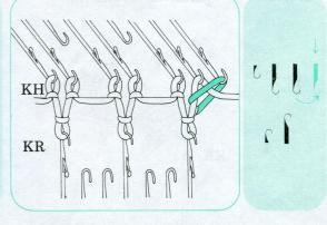
L-1)-b Knit 2 rows and rack. Take the loop of edge stitch on KH and transfer it onto the 3rd empty needle on KR. (By operations (a) and (b) 1 stitch is increased.)
