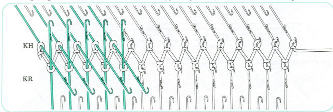
③Knit 1 row. The yarn rests along the needles in E position on both KH and KR. Put yarn behind the innermost needle on KR which is in E position.
