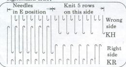
③ As illustrated by the diagram hook the yarn on the needle marked 1. Set the carriage for "PART" and pass the carriage to the righthand side.
