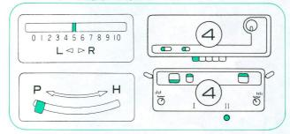
To work tuck stitches on Push Button Machine With KH-588 and KH-710 push button machines, push end needle to E position.
