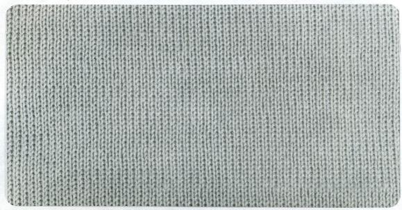
Full-needle rib is worked using every needle on KH and KR. Half pitch lever to H. The stitches are very close together and have high elasticity. They are widely used for collars, cuffs, etc.
