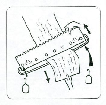
The edges of ribbed knitting are apt to stretch so reducing the effect of the weights. Symptoms of this are dropped or badly knitted stitches. To prevent this, use a small weight with an L-shaped wire weight hanger or a claw weight to hold your knitting down. Re-position these edge weights every 30 - 35 rows, or as needed.
