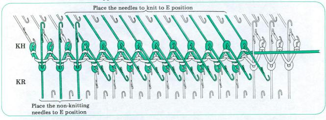
(4) Knit 1 row to the left. Pass the yarn behind the innermost non-knitting needle in E position on KR.
