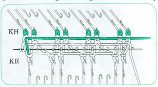
$\bigcirc$  After working the finished edge cast-on with circular knitting, reset the machine as the diagram below and continue knitting  $2 \times 2$  ribbing.
