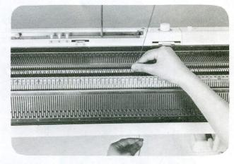
② Thread the yarn into the yarn feeder. (See instruction manual accompanying Ribber attachment)
