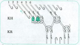
(4-a) Knit until the next decrease. Transfer the 6th stitch onto the 5th needle and move in the double stitch to the 6th needle.
