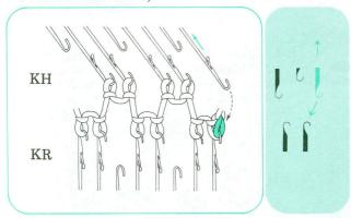
3 Continue knitting until next decrease, Transfer the edge stitch onto the adjacent needle on KR. Push back the empty needle to A position.
