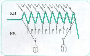
★ When you work tucked rib patterns use the wireloop type weight hanger on each side.
