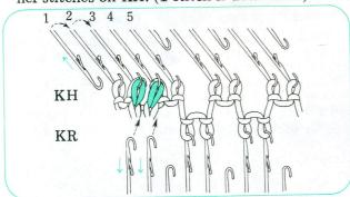
②-a) Knit until the next decrease. Transfer the 4th stitch on KH onto the 3rd stitch and move the double stitch back to the fourth needle.
