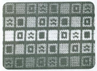
For multi-coloured rib patterns, punchcards, pattern card and colour changer are used. Unlike coloured patterns worked on KH alone, there are no yarn floats on the wrong side, so the appearance is very neat on either side.
