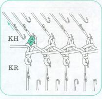
the edge stitch onto the inner needle. Push back the empty needle to A position. (1 stitch is decreased.) Racking Indicator 5
