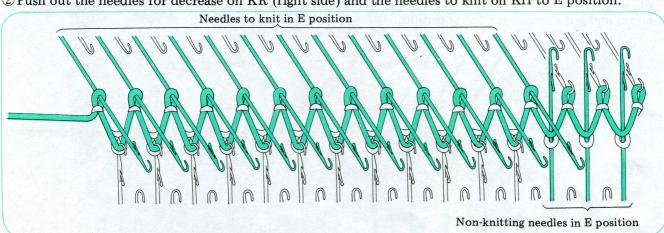
③Knit 1 row from left to right. Pass the yarn behind the innermost non-knitting needle on KR. Push up the needles for decrease at the opposite side on KR and the needles to knit on KH to E position.
