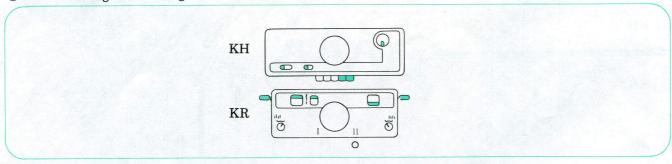
2 Push out the needles for decrease on KR (right side) and the needles to knit on KH to E position.
