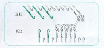
B-2) Move the carriage once. The needles arranged in B position catch yarn, Hang the wireloop type weight hanger and a small weight.
