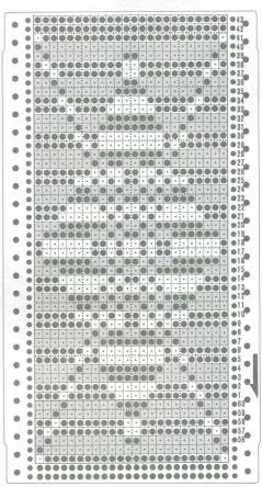
The bassic card on the left shows the pattern repeated twice. The RevisedCard above shows only one pattern due to the fact that each row is punched twice (once for the main colour and once for the contrast colour).
