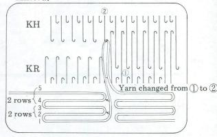
With the above operations 1 buttonhole is completed. Set the carriages for ribbing and continue knitting until the next buttonhole position.
