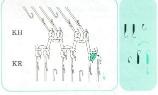
④ Knit 1 row. Transfer the first stitch on KR onto the needle on KH and push back the empty needle to A position. (By operations (3) and (4) 1 stitch is decreased).
