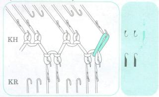
(4) Knit until the next increase. Take the loop of the first stitch on KH and transfer it onto the next vacant needle. (1 stitch is increased.)
