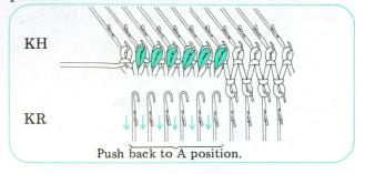
C) 2×2 rib (Half pitch lever on H)
