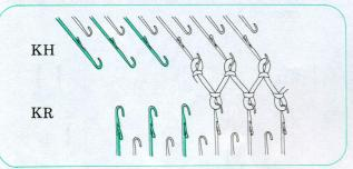
A-2) Move the carriage once over the needles. The needles arranged in B position catch yarn. Hang a wire-loop type weight hanger and a small weight and continue knitting.
