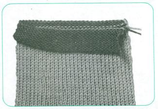
Though the way of finishing off the ribbed stitches is just the same for both single and double bed machines, with the KR the purl stitches and plain stitches are clearly distinguished if they are separated by circular or U-style waste knitting. You can then fold down the waste knitting and finish the edge by hand as shown.
