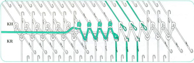
©Knit 1 row to the right. Pass the yarn behind the stem of the first needle in E position, and at the opposite side to the carriage, push back the needles on KH to D position. On KR, put back stitches into the hooks and push them back to B position.
