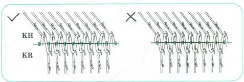
②Knit 8-10 rows. Drop all the stitches off KR. Push back the needles on KR to A position. Knit 1 row on KH only using cast-on thread.
