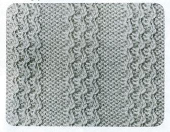
Above pattern stitches are worked by racking the KR machine 2 pitches in alternate directions. This makes a very interesting textured pattern.
