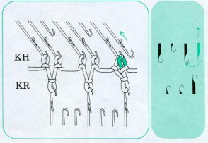
R-1)-b) Rack first. Then transfer the edge stitch on KR onto the inner stitch. Push back the vacant needle to A position. (By operations (a) and (b) 1 stitch is decreased.)
