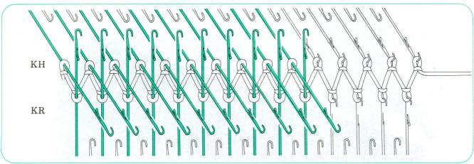
③ After knitting a row, the knitting yarn rests along the KH and KR needles in E position. Put yarn behind first held needle on KR.
