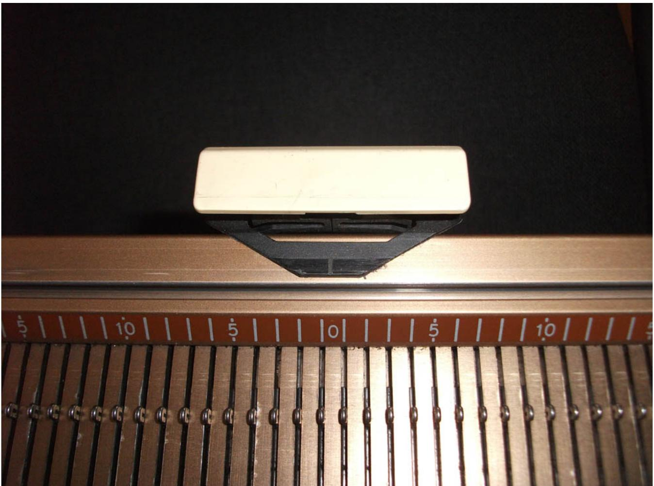
It may be needed to reset the start position of the cursor, like in: you need to unravel one or more rows after a jam. You normally position the carriage outside the knitting area, move the cursor from right to left in one go and stop opposite the 0 mark on the needle bed, press the "Pos 0" button and move the cursor to the side where the carriage is.
